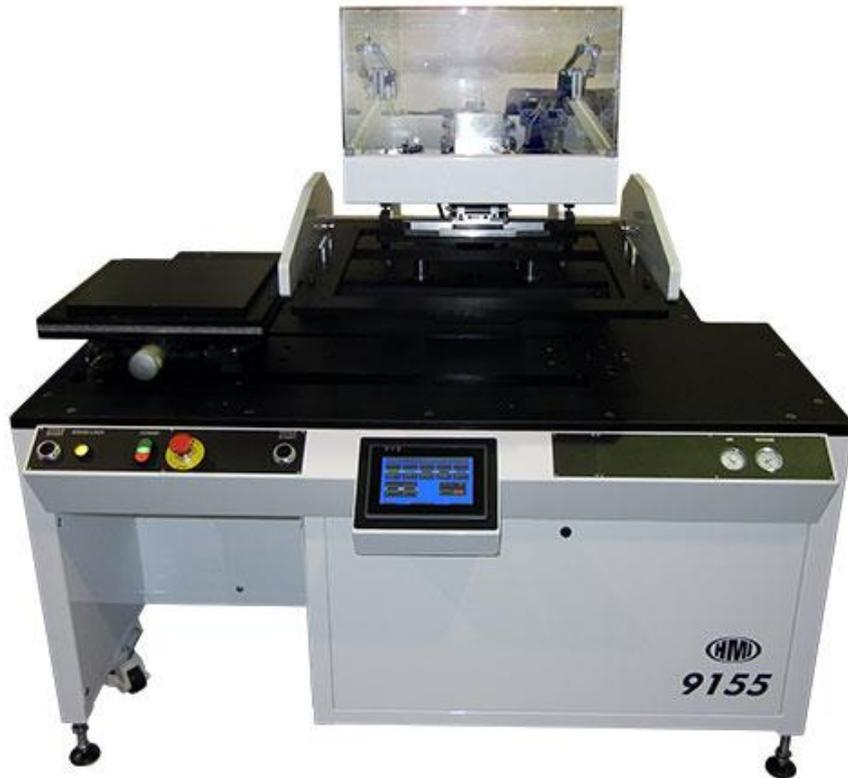
**The MSP-9155 is a semi-automatic screen printer designed for large area print applications that require a high resolution, reliable result.**
