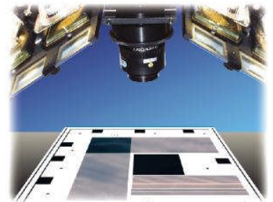
Inspection Calibration Standard
